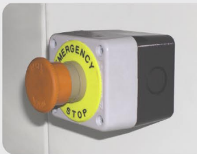
後部緊急開關 (後面收料人員, 可控制機械而減少不必要之損失) Emergency switch on the machines rear. (the emergency to stop working decision depend on rear operator. It can decrease lose when improper control.)
