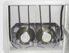
機械碟式煞車裝置 Disc braking mechanism.
