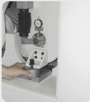
快速更換裝置 Quick replace sanding belt device.
